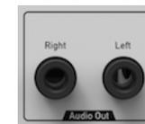
The KB37 features a stereo signal path which is also buffered by an output stage. Even when you're using a mono setup within your module patches, it's not a bad idea to do a 2-channel connection to your mixer. As long as you use the Left / Mono In jack only on the front panel, the signal is sent to both outputs. This way you can switch between mono and stereo output quickly by just inserting a patch cable.
